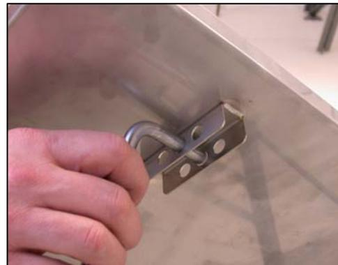
Figure 1-6. Drain tray hook.
