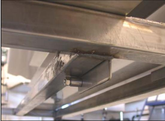
Figure 1-7. Bucket support fasteners.
