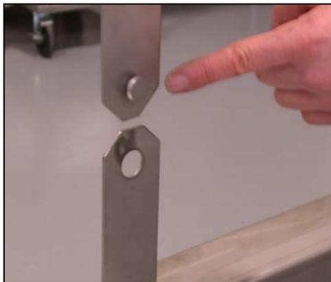
Figure 1-4. Applicator frame connector.
