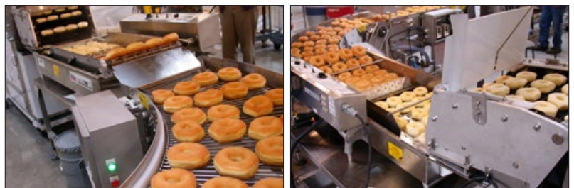
Below: Century - Mark VI system in operation. Frying and proofing functions are synchronized.
